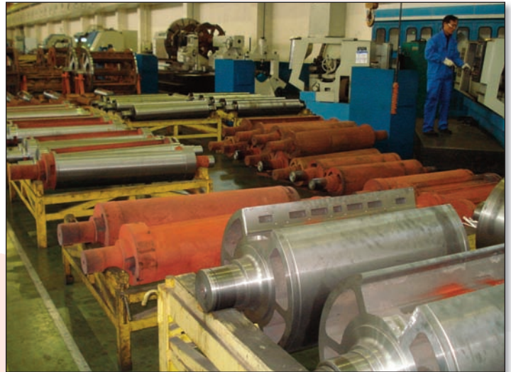
Press cylinders in various stages of production at Guanghua.
